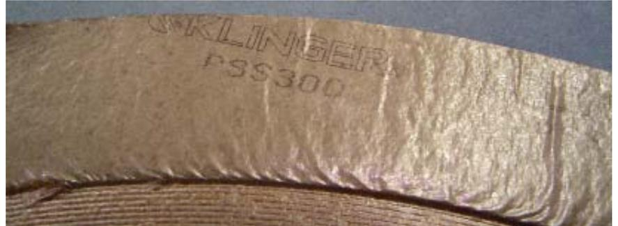
*The spent gaskets (pictured) showed no signs of deterioration caused by media or high temperature and were acclaimed by mechanical staff for their ease of removal. Milam has also proved to be a robust material resistant to the ill effects of manual handling. The customer was said to be impressed by Milam's quality of con-*
