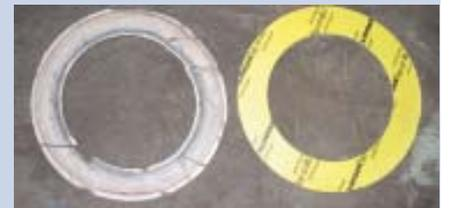
*The gasket remained tight throughout its entire working time and developed no functional problems. It was removed solely in order to document its condition after one year of operation. During removal, the gasket was easy to separate from the flange faces, with no sign of adhesion. In fact, it was still possible to discern the gasket's KLINGER® top-sil ML1 lettering. A new KLINGER® top-sil ML1 gasket was immediately fitted in its place.*
